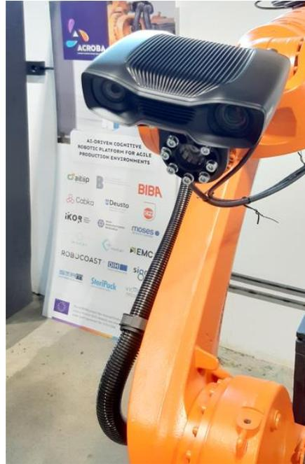
**Figure 10 Zivid Two Camera onboard the robot.**
