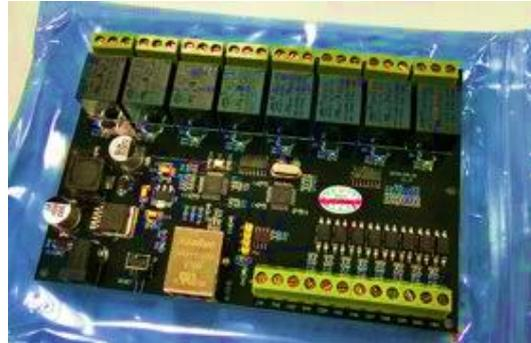
Figure 10: TCP/IP board.
