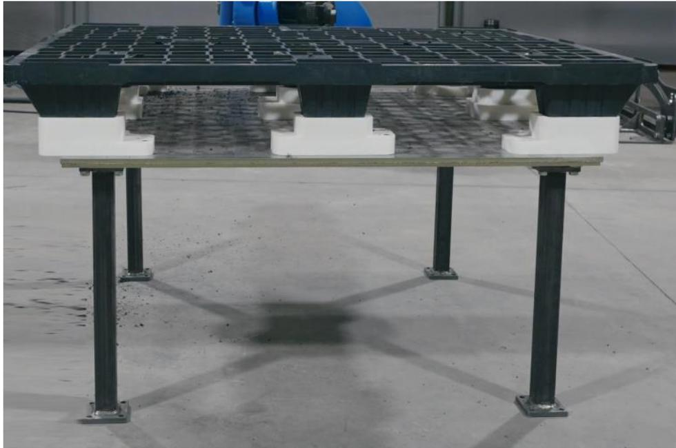
Figure 15 : Workbench for the deburring
