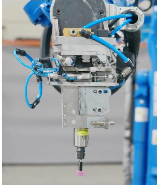
Figure 16 : Milling tool for the deburring
