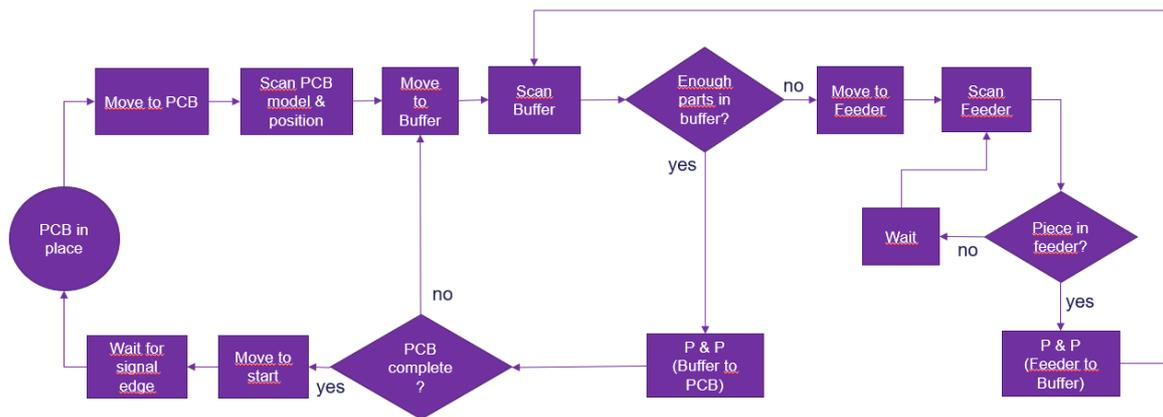
**Figure 53 Diagram of IKOR's Sequence**
