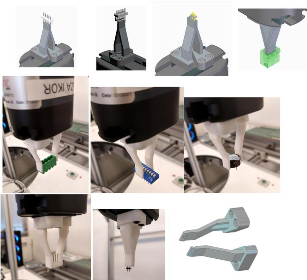
**Figure 45 Images of the final design created at IKOR to handle electronic components**
