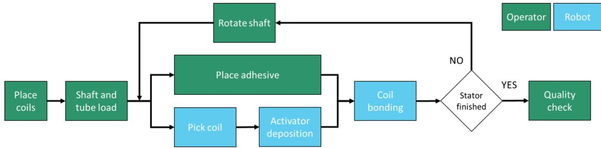
**Figure 57 Flowchart of the high-level order of tasks of the Coils bonding process**
