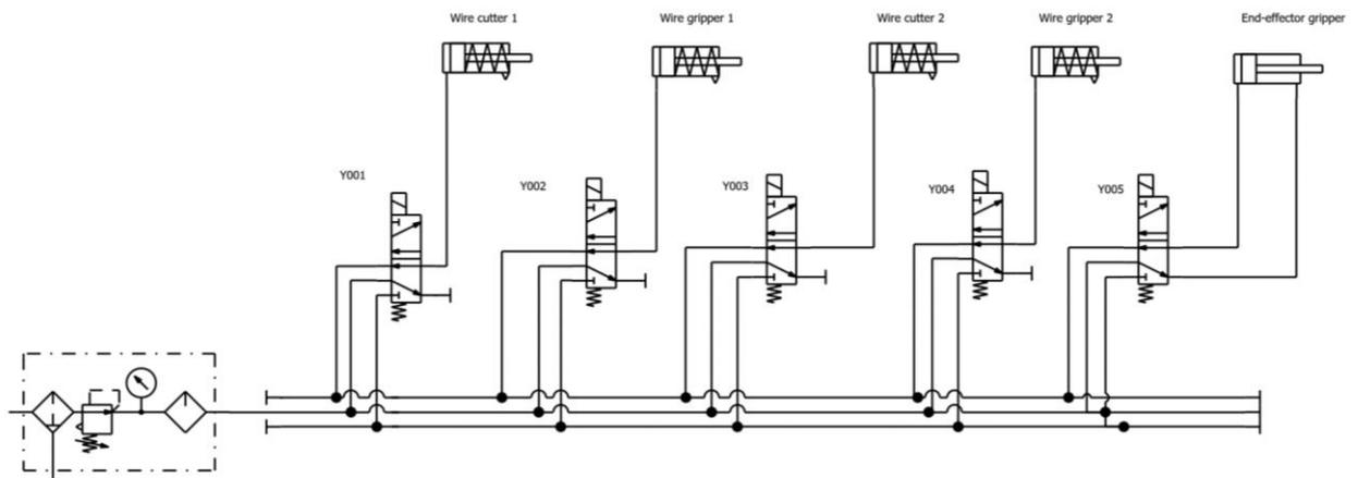
**Figure 33 Winding cell pneumatical scheme**
