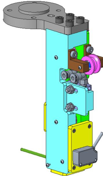
**Figure 29 Winding end-effector**
