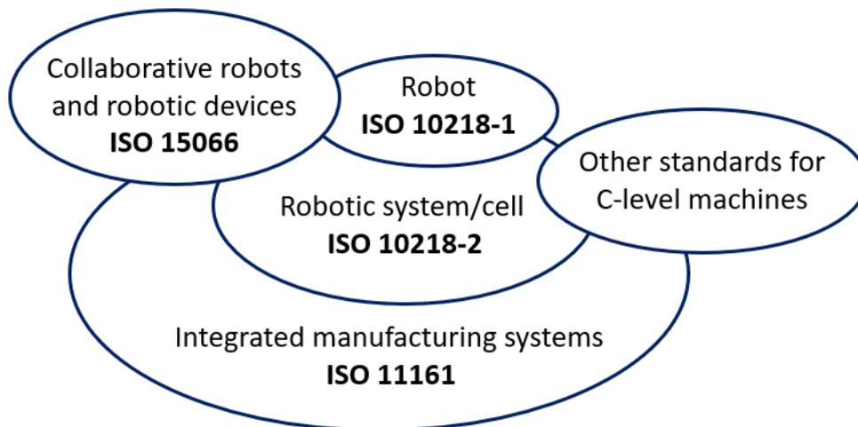
**Figure 19 Diagram of relationships between standards for collaborative robotic system**
