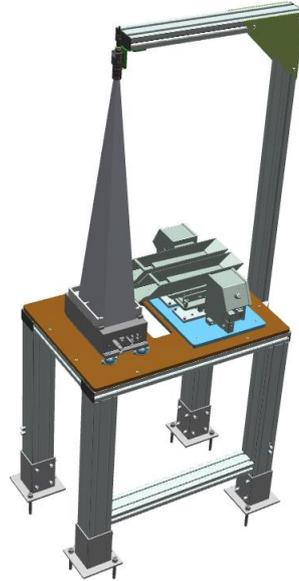
***Figure 7 Vibrating Table 3D View***
