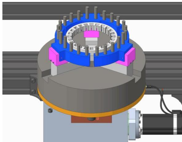
**Figure 30 Metal pins to hold the wire**
