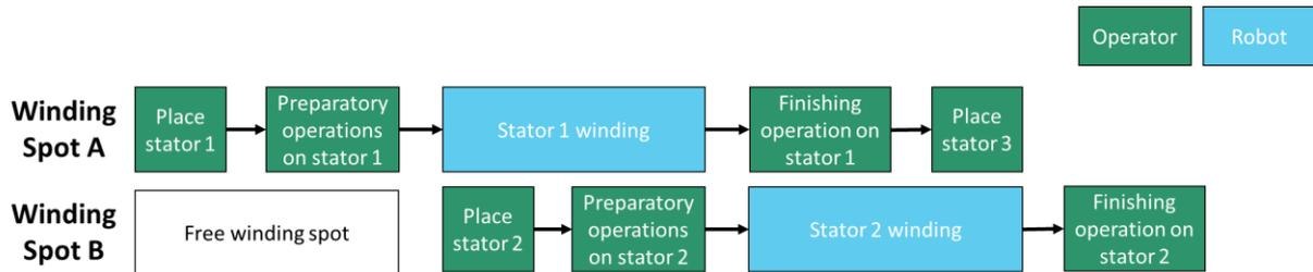
**Figure 54 Flowchart of the high-level order of tasks of the Coils winding process**
