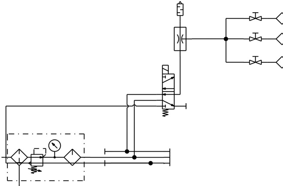
**Figure 38 Bonding cell pneumatical scheme**
