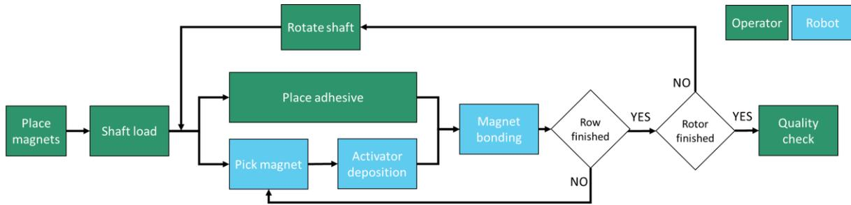
**Figure 56 Flowchart of the high-level order of tasks of the Magnets bonding process**
