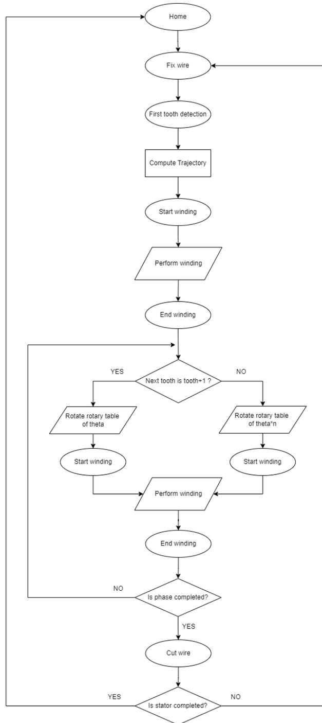
**Figure 55 Stator winding flowchart**
