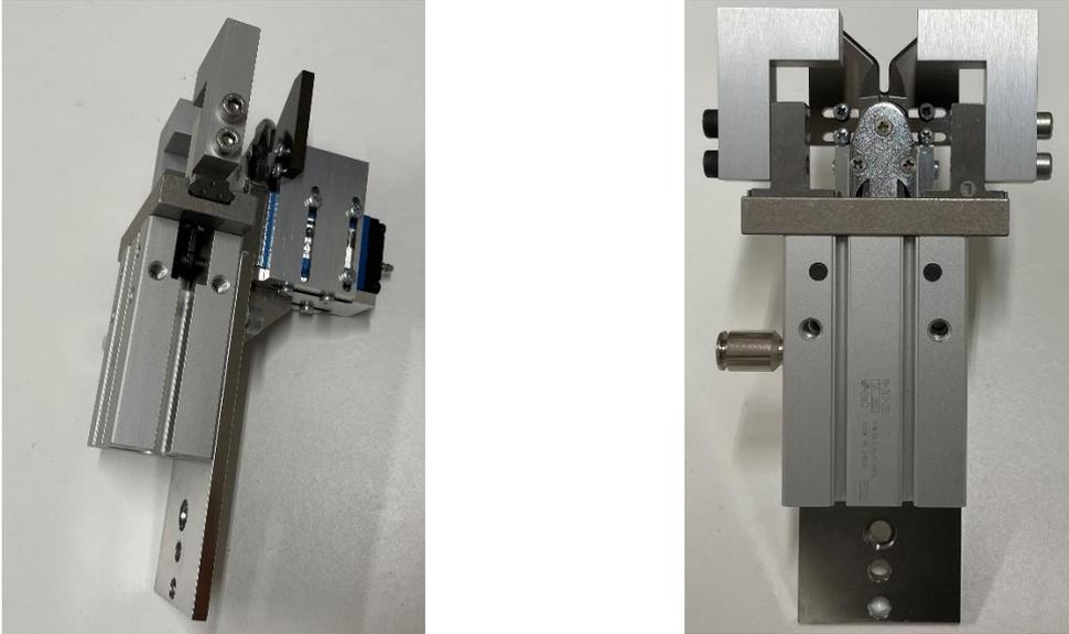
**Figure 50 Tool for wire cutting operation.**
