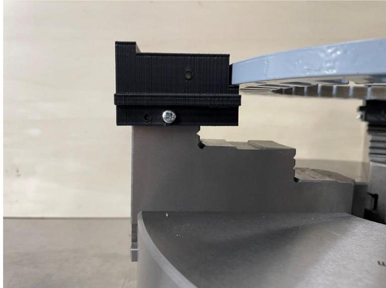
**Figure 28 3D printed finger**
