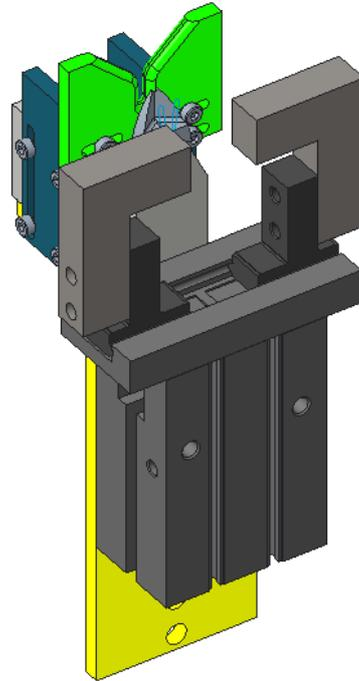
**Figure 32 Tool for wire cutting**
