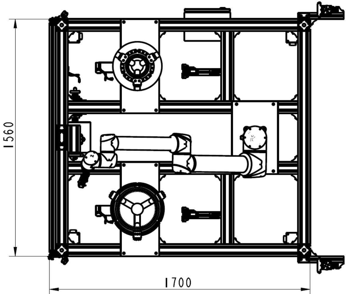
*Figure 24 Winding cell layout*
