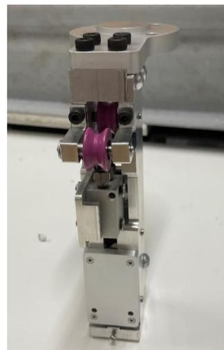
**Figure 49** winding end-effector
