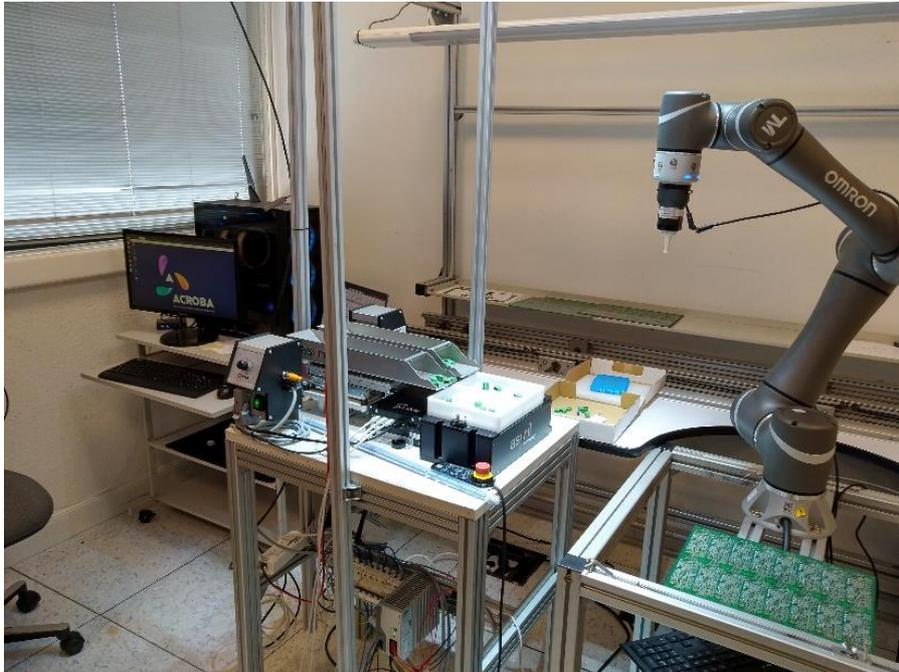
**Figure 46 Image of the provisional robotic cell created at IKOR**
