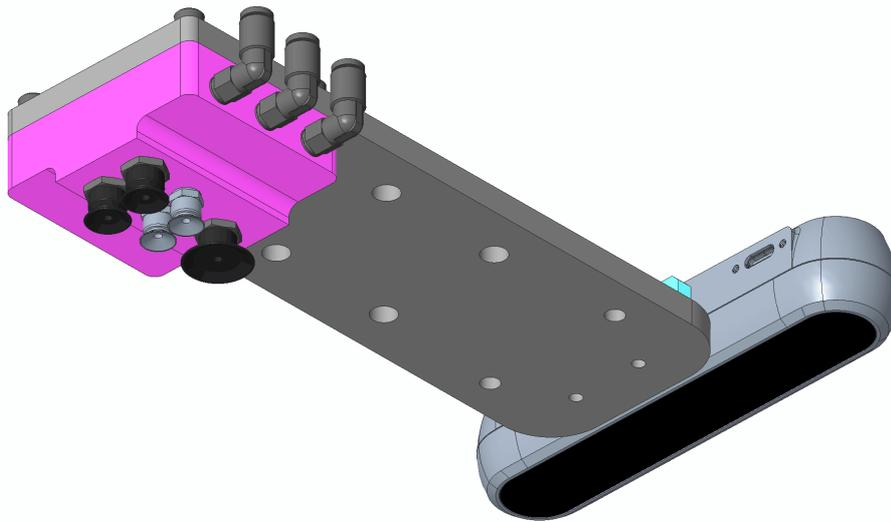
**Figure 37 Bonding end-effector**
