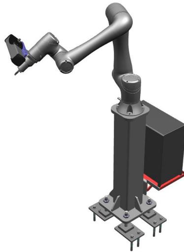
***Figure 9 Cobot's Base 3D View***
