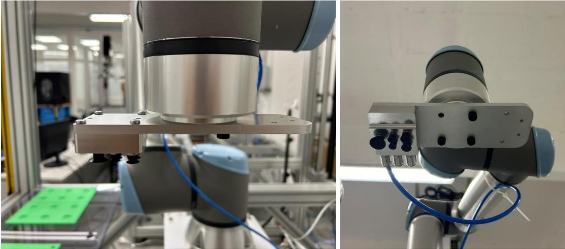
*Figure 76 – ICPE bonding end-effector*
