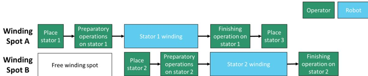
Figure 82: Flowchart of the high-level order of tasks of the Coils winding process
