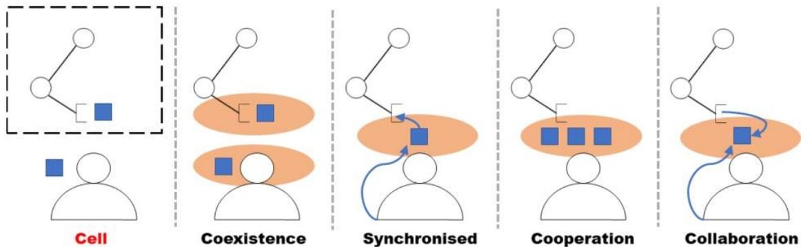
Figure 2: Classification of methodologies for human-robot shared working space
