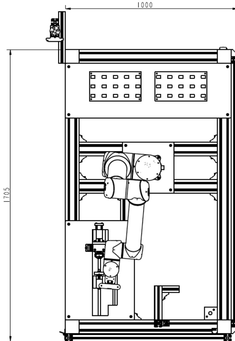
*Figure 44: Bonding cell layout*
