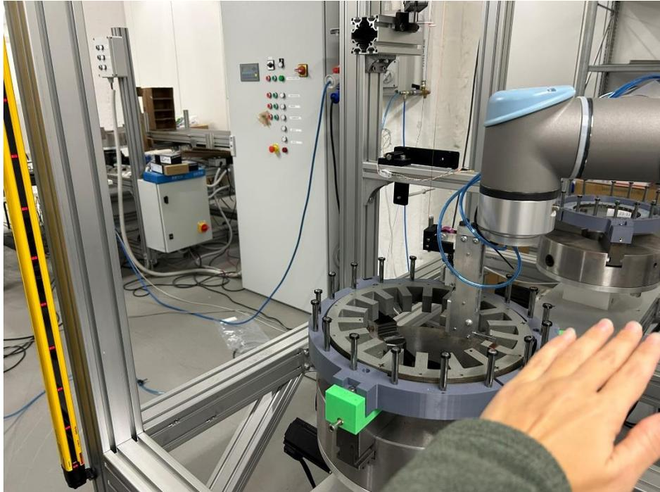
*Figure 71 - ICPE winding safety light curtain (red mode)*
