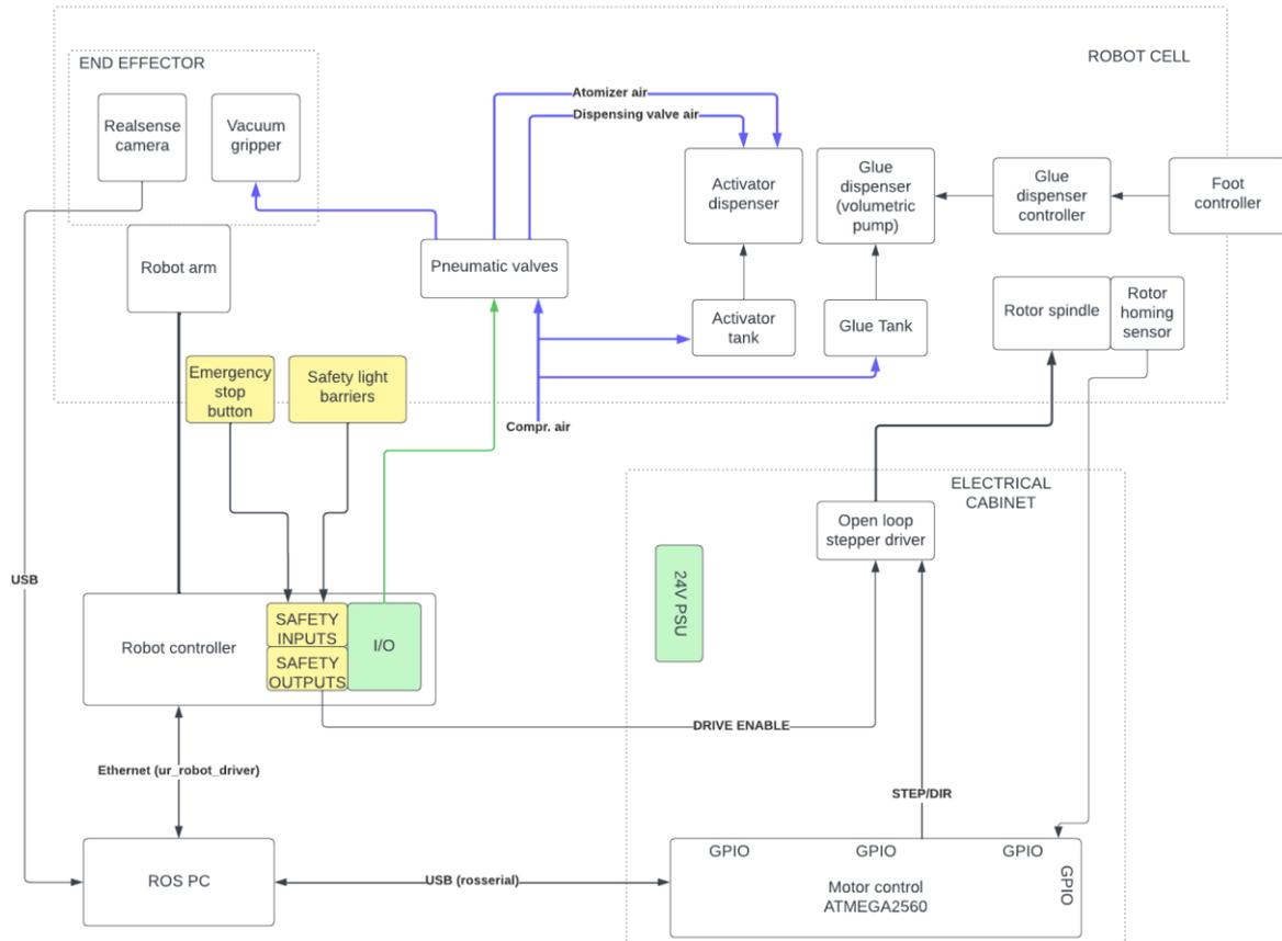
Figure 50: Bonding electrical design
