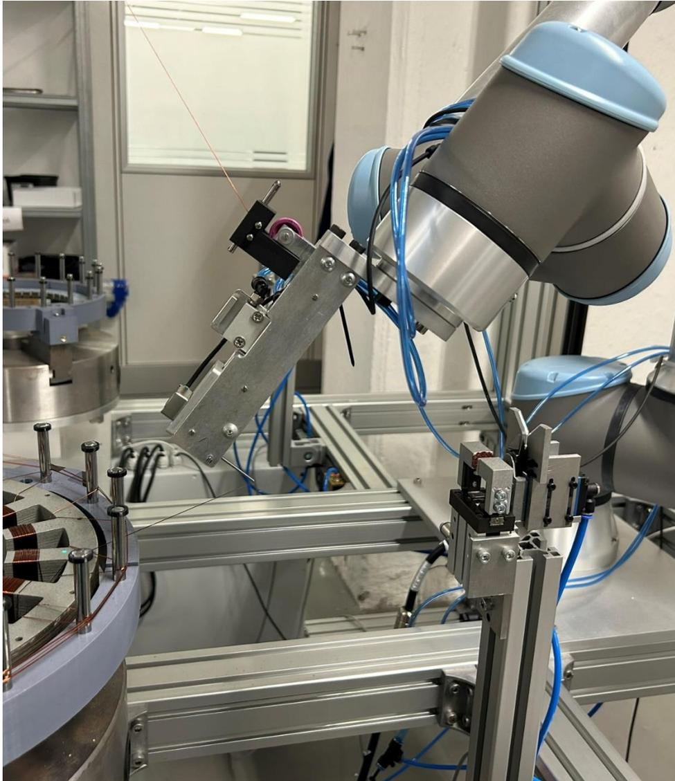
*Figure 65 – ICPE winding end-effector*
