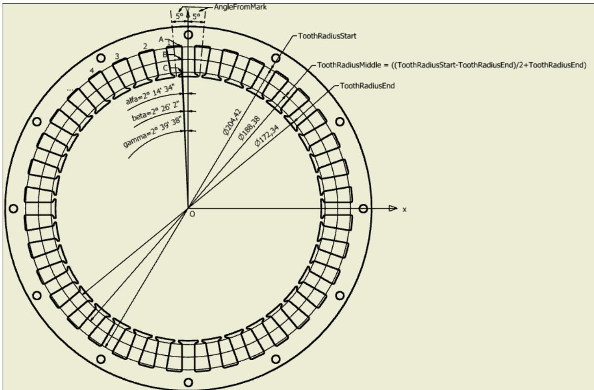
Figure 91 - Angle from mark. Angle between slots. Tooth edge angles - measured on 3D model.
