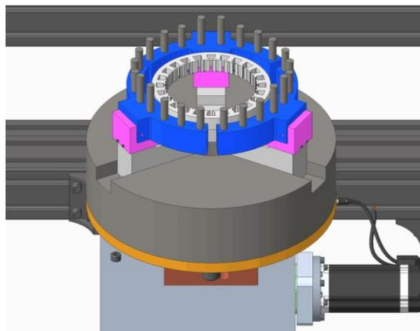
*Figure 40: Metal pins to hold the wire*
