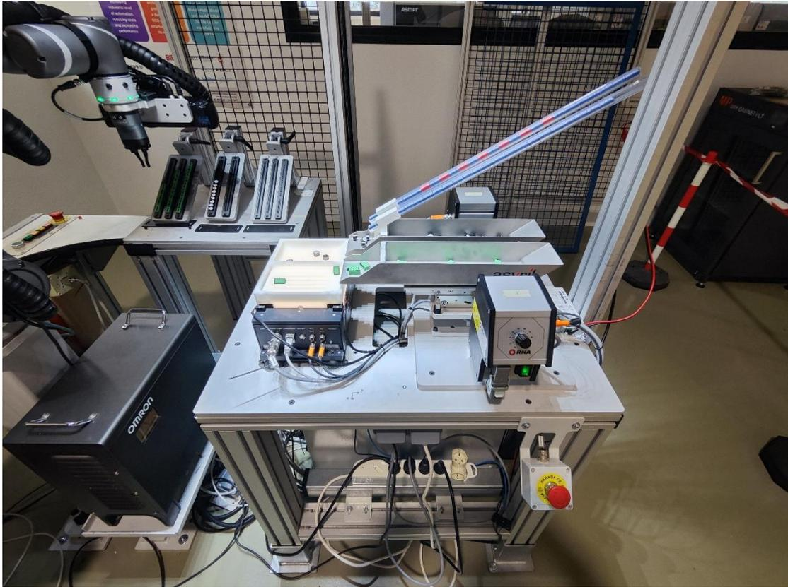
*Figure 61: View of the rest of the main elements: vibratory system and intermediate surface*
