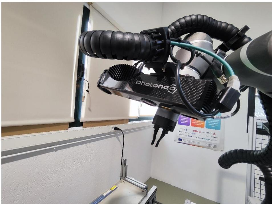
*Figure 18: Detail of the final tool of the robot and the Photoneo Vision System*
