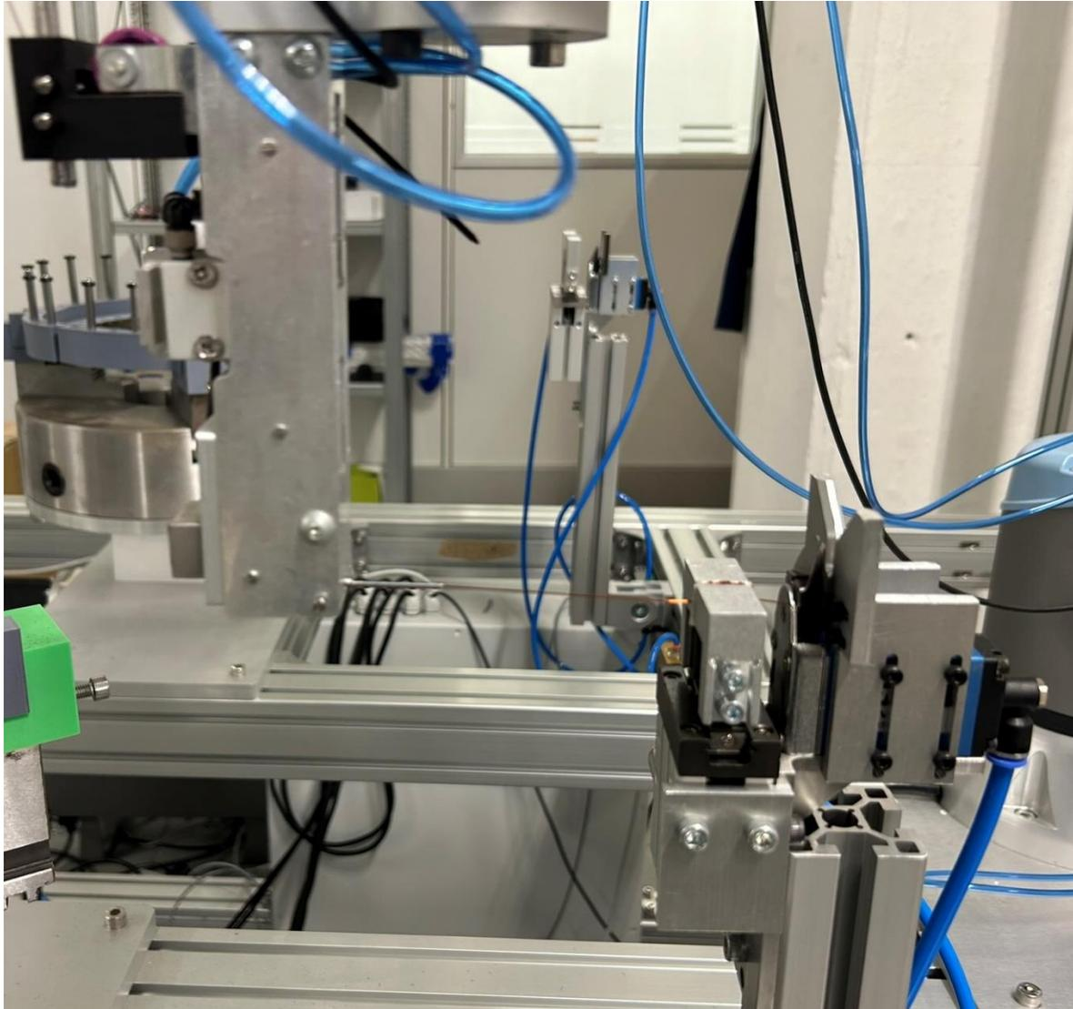
*Figure 66 – ICPE winding pincher*
