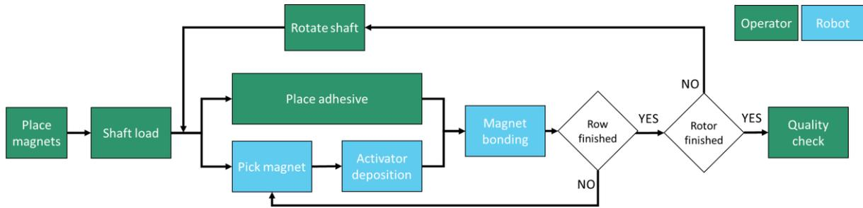
Figure 83: Flowchart of the high-level order of tasks of the Magnets bonding process
