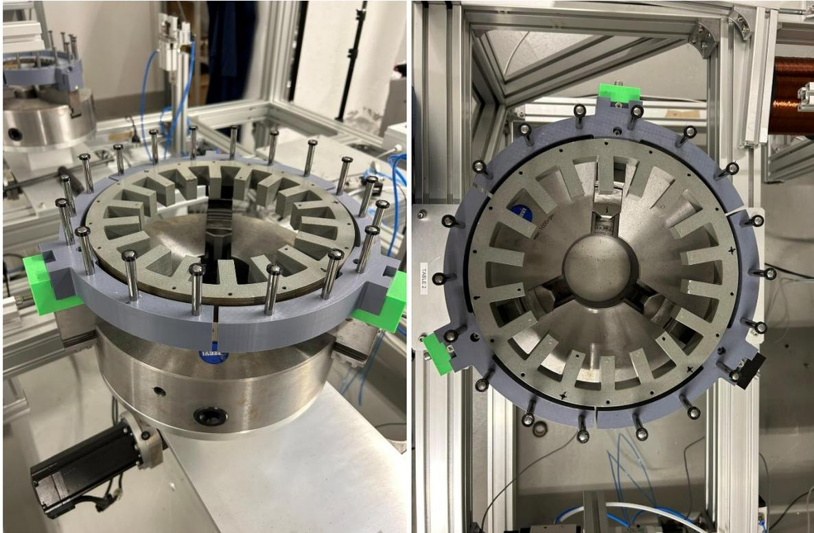
*Figure 68 – ICPE winding rotary table*
