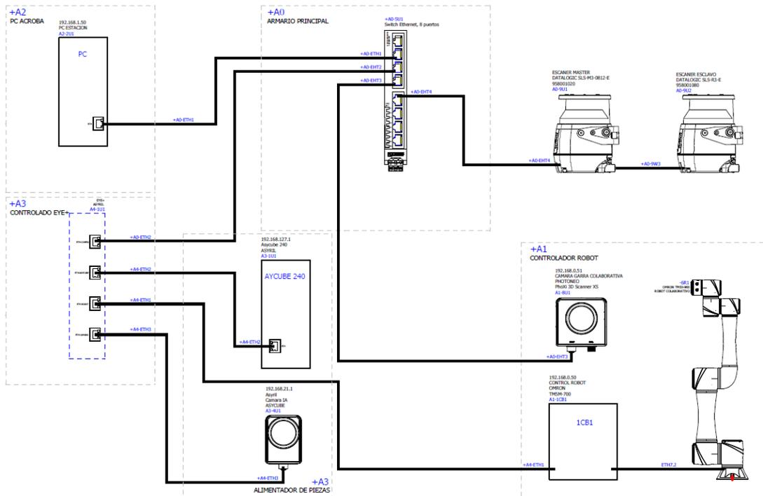
Figure 19: IKOR'S control architecture including scanners
