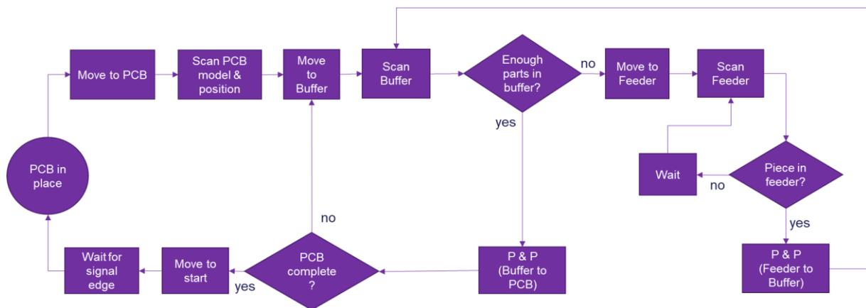
Figure 7: Sequence diagram for IKOR's use case
