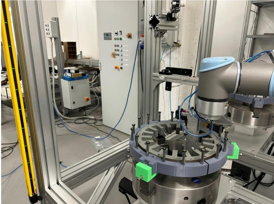
*Figure 70 – ICPE winding safety light curtain (green mode)*
