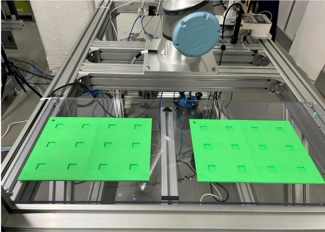
*Figure 75 – ICPE bonding trays*
