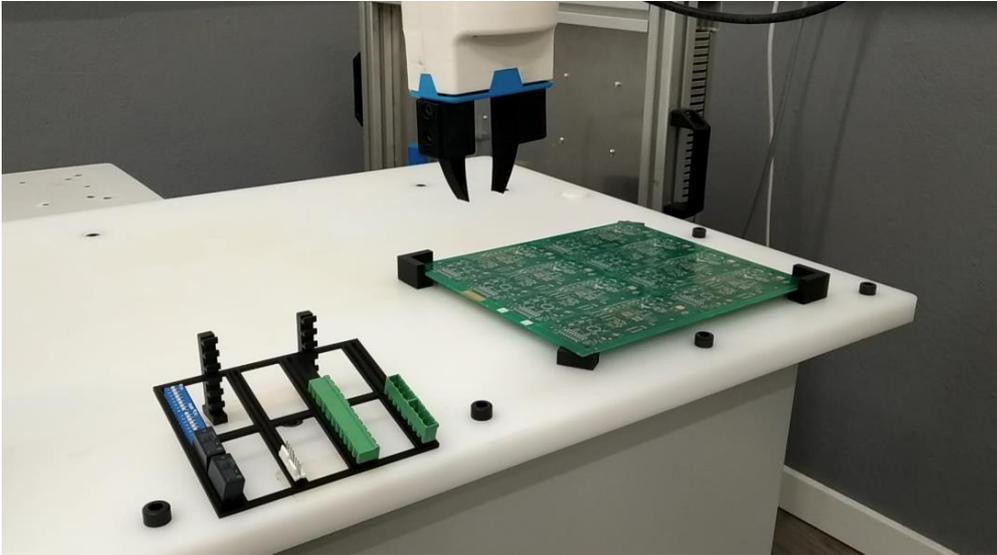
*Figure 4: Preliminary Pick and Place test in NUTAI*
