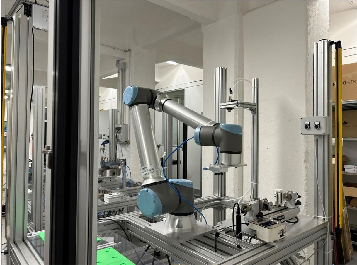
*Figure 74 - ICPE use case bonding cell*
