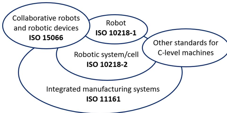
Figure 23: Diagram of relationships between standards for collaborative robotic system
