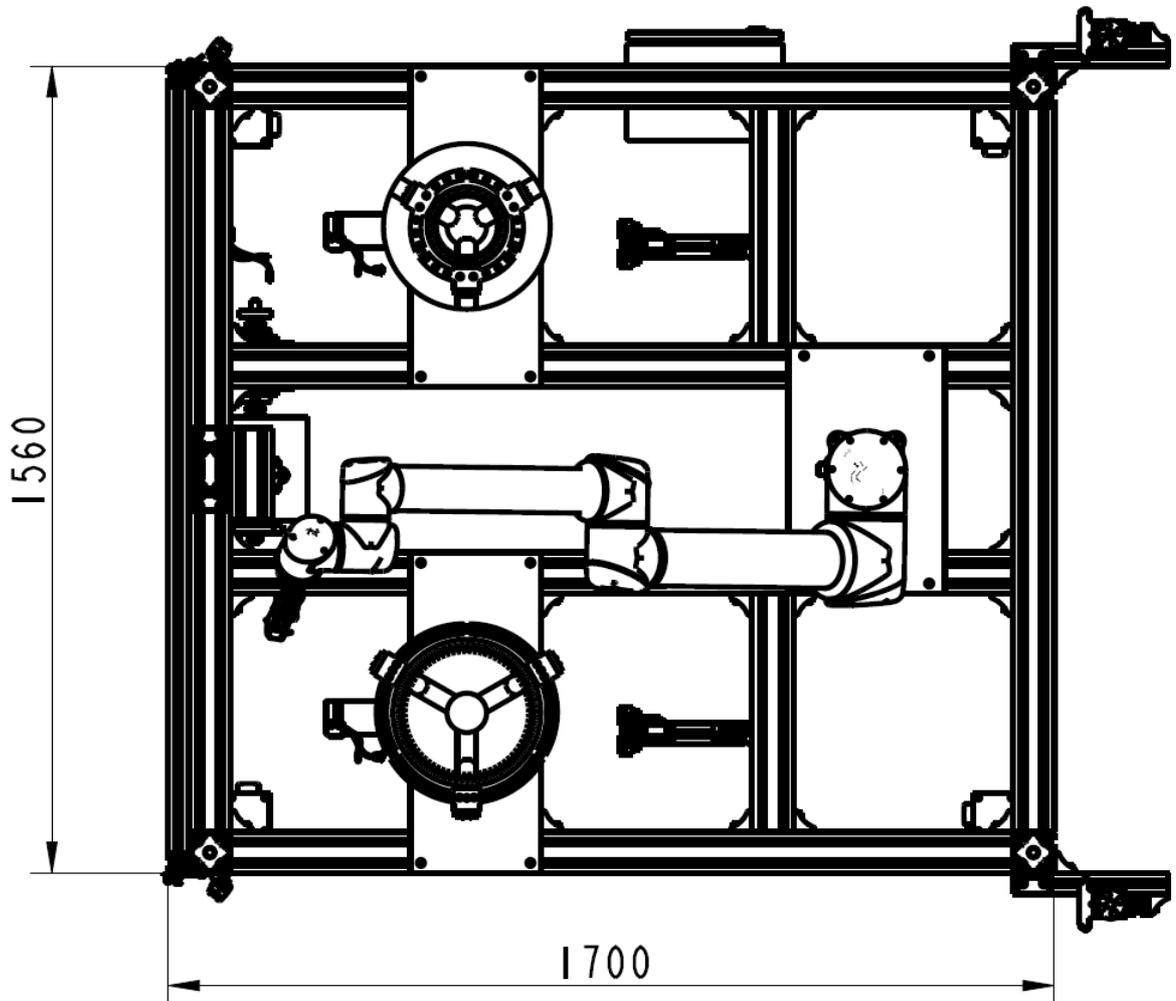
*Figure 34: Winding cell layout*
