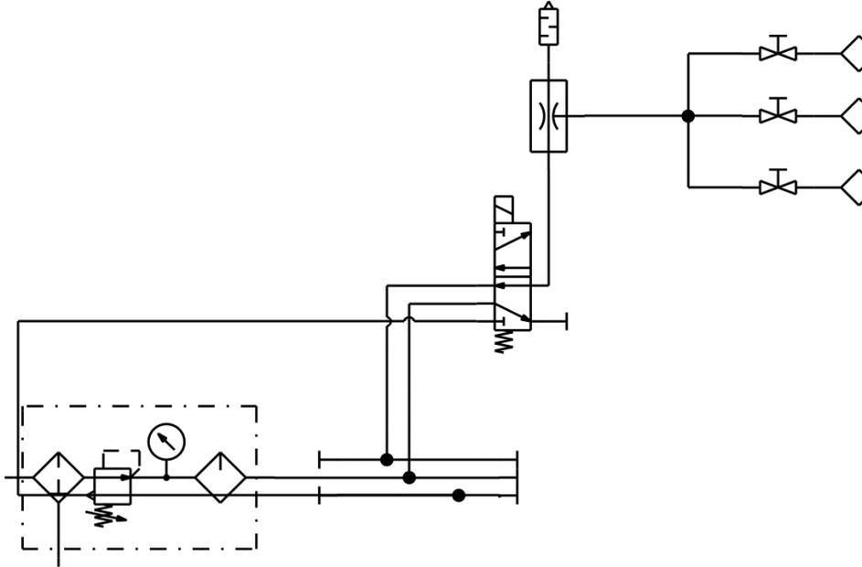
Figure 48: Bonding cell pneumatical scheme
