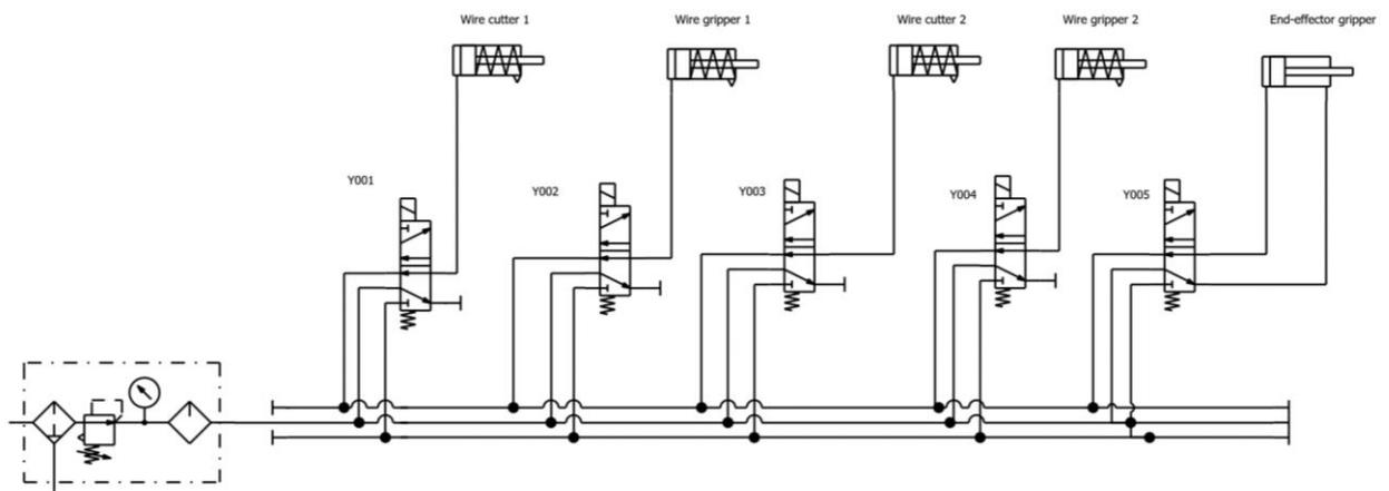
Figure 43: Winding cell pneumatical scheme
