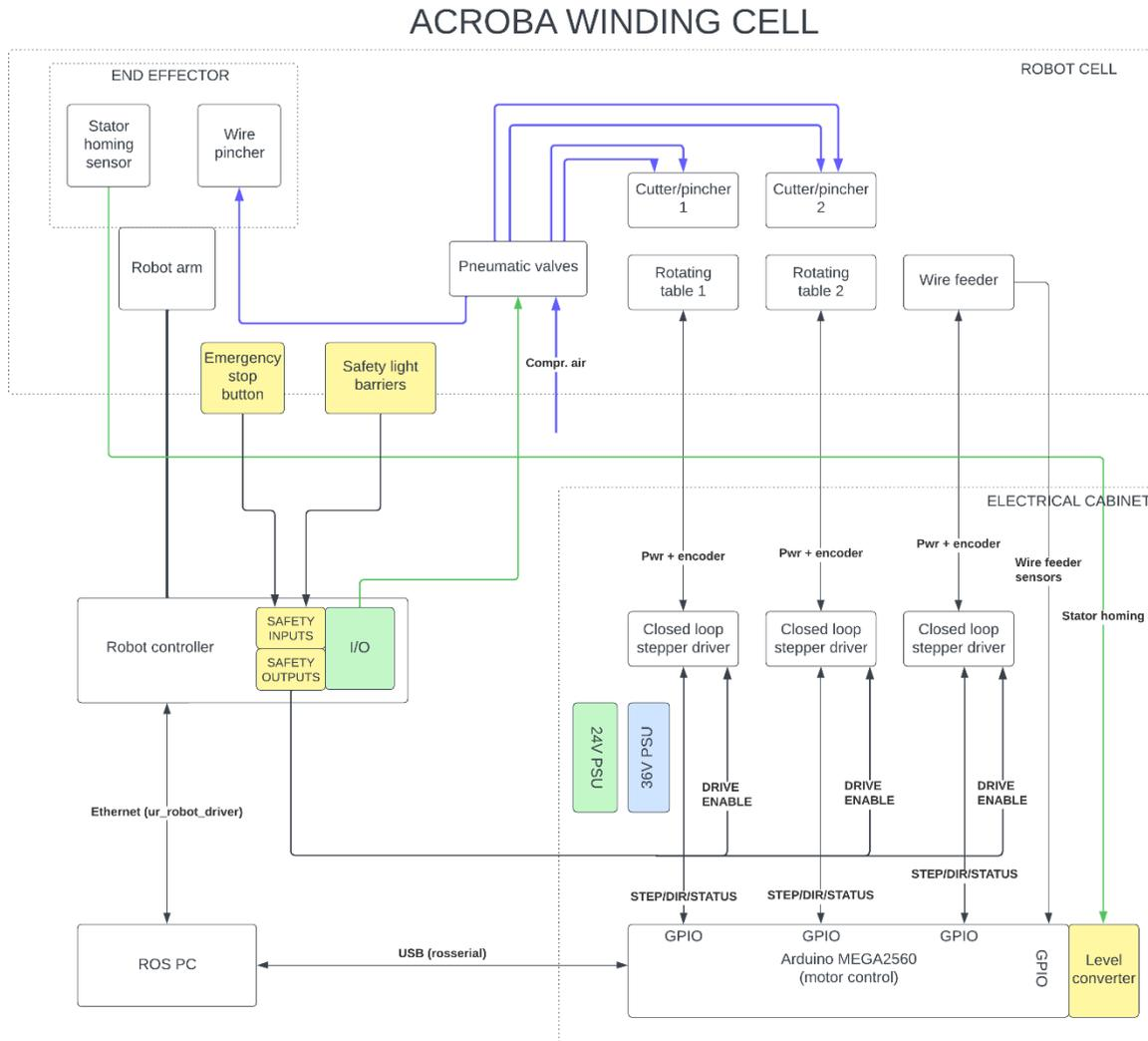
Figure 49: Winding electrical design
