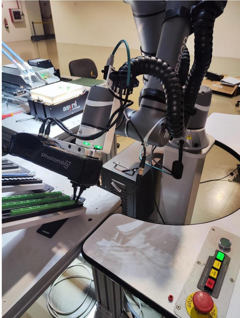
*Figure 62: Detail of the robot picking a component*
