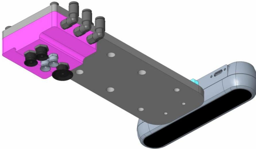
*Figure 47: Bonding end-effector*
