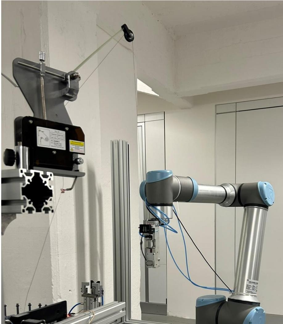
*Figure 69 – ICPE winding tensioner*
