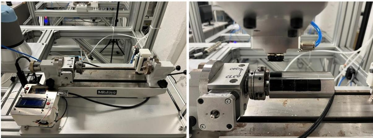
*Figure 77 – ICPE bonding spindle*
