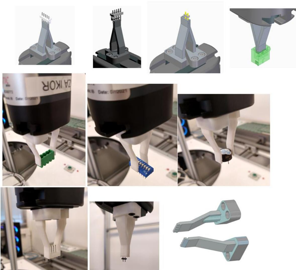
*Figure 57: Images of the final design created at IKOR to handle electronic components*
