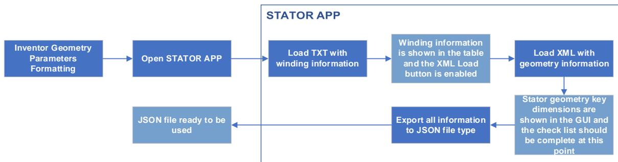
Figure 92 - Generating Stator Winding json file
