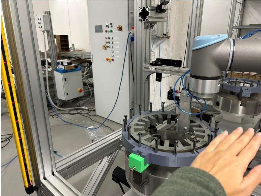
*Figure 25 - ICPE winding safety light curtain (red mode)*
