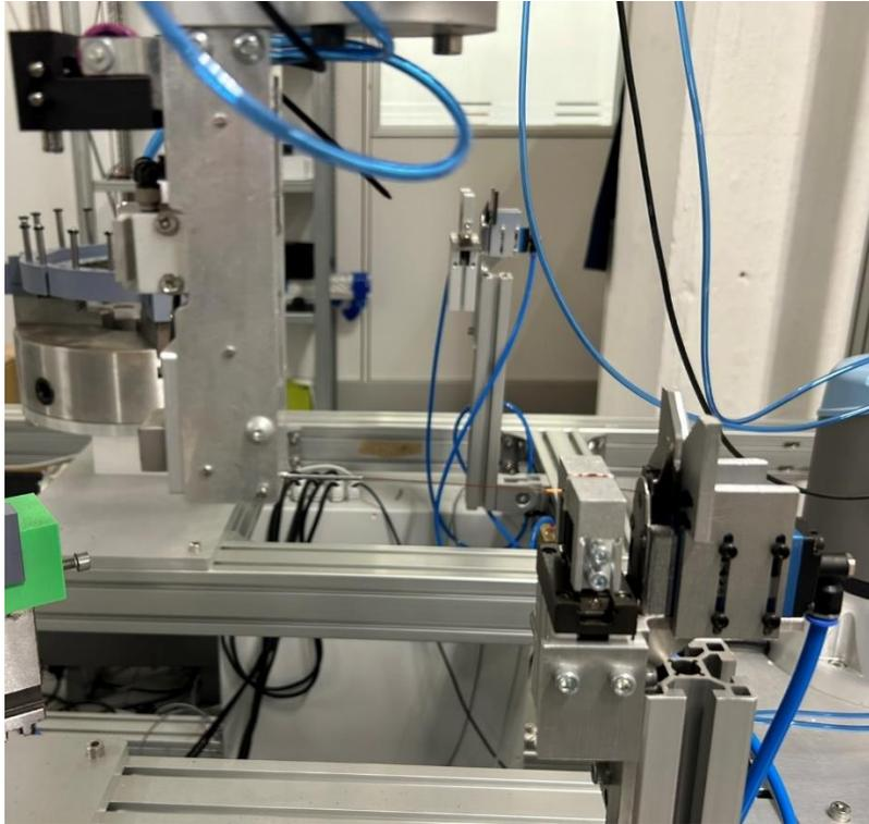
*Figure 30 – Wire fixed into the pincher*
