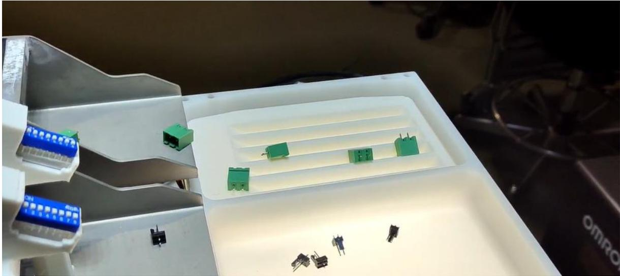
*Figure 14: Green 2 pin components in the feeder*
