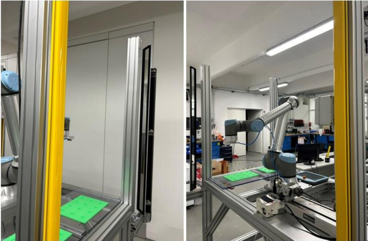
*Figure 26 - ICPE bonding safety light curtains*
