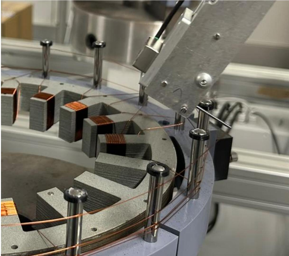
*Figure 33 - Detail of stator outer pins*
