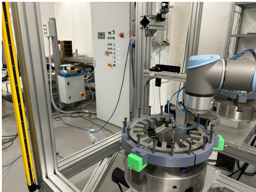
*Figure 24 - ICPE winding safety light curtain (green mode)*
