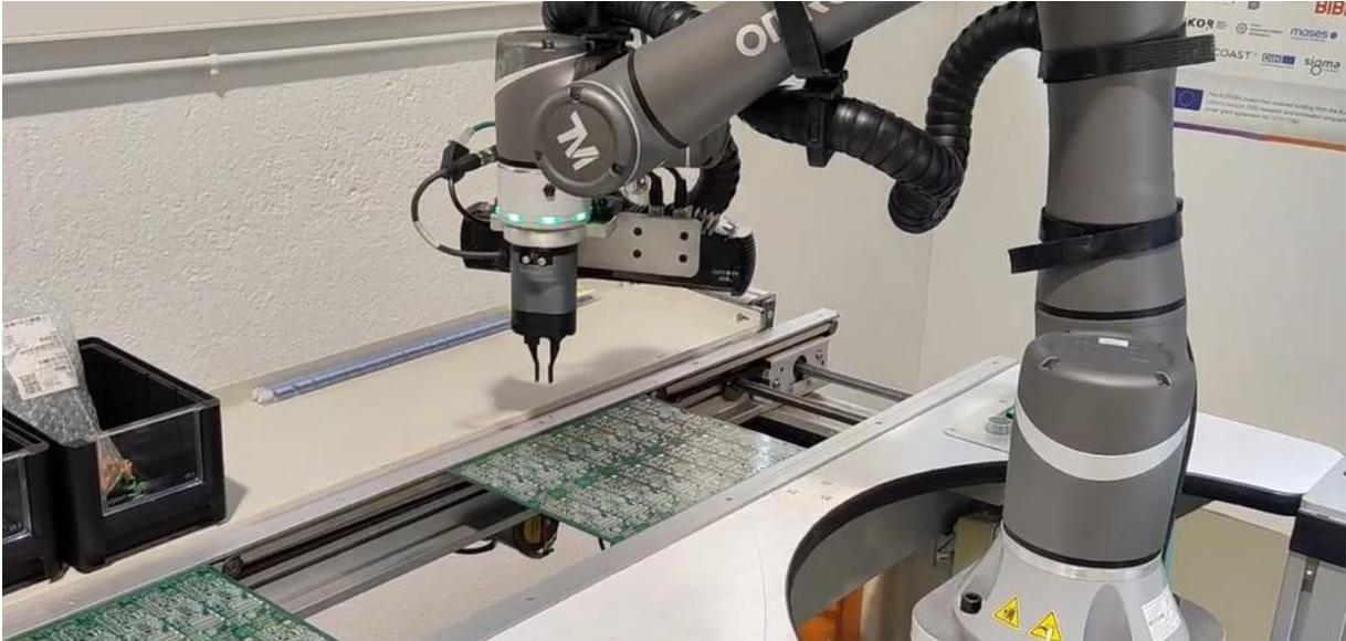
*Figure 18: Robot movement to PCB scanning pose*
