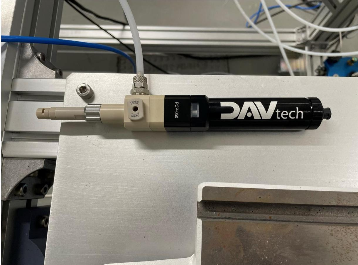
*Figure 40 - Volumetric pump for glue dispensing*
