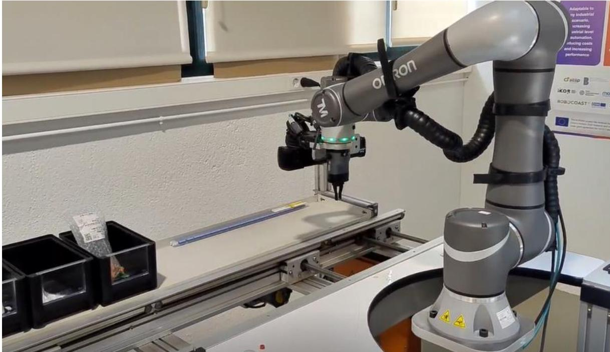
*Figure 17: Waiting pose when no PCB is detected*
